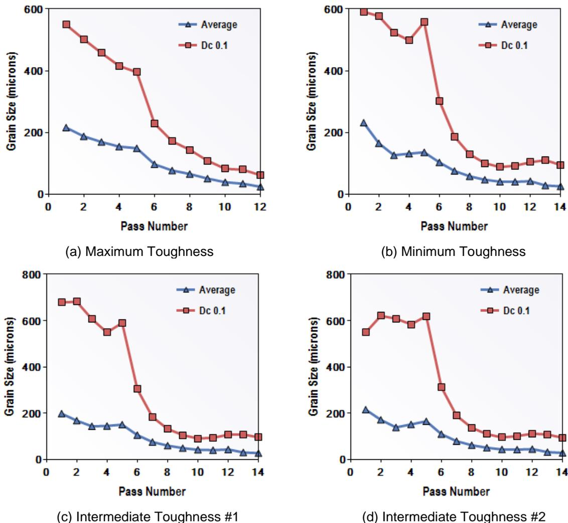
**Figure 3.** Average and  $Dc_{0.1}$  grain size of austenite along the pass schedules of the 10 mm NR plates studied in this paper, as calculated by MicroSim®.
