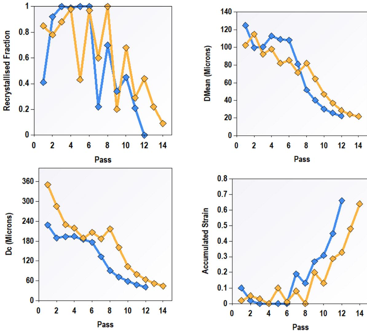
**Figure 7.** Several austenite microstructural parameters got along the pass schedules of the 30 mm NR plates studied in this paper, as calculated by MicroSim®. The blue line indicates the good toughness plate, while the yellow one indicates the fair toughness plate. The number of roughing passes was 6 for the good toughness plate and 8 for the fair toughness plate.
