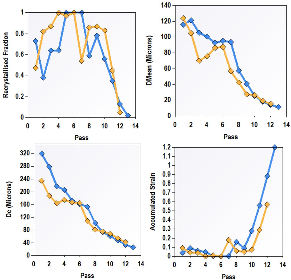
**Figure 5.** Several austenite microstructural parameters got along the pass schedules of the 15 mm NR plates studied in this paper, as calculated by MicroSim<sup>®</sup>. The blue line indicates the good toughness plate, while the yellow one indicates the fair toughness plate.
