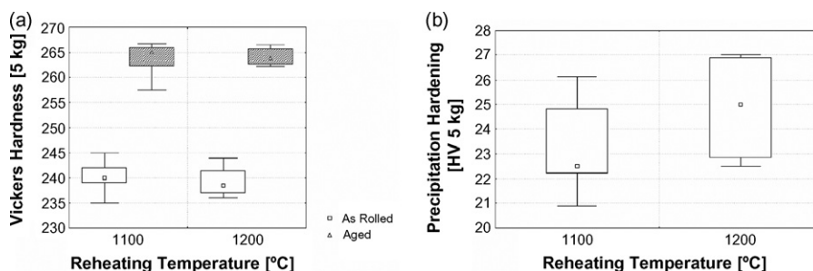
Fig. 1 – Reheating temperature effect over (a) as-rolled and aged hardness and (b) precipitation hardening.
