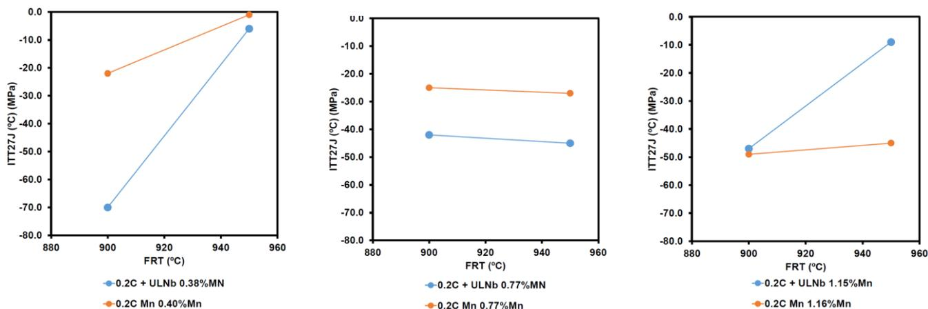
**Figure 6:** Effect of finish rolling temperature on impact transition temperature at 27 J for CMn (Group A) and ULNb (Group B) steels [11].
