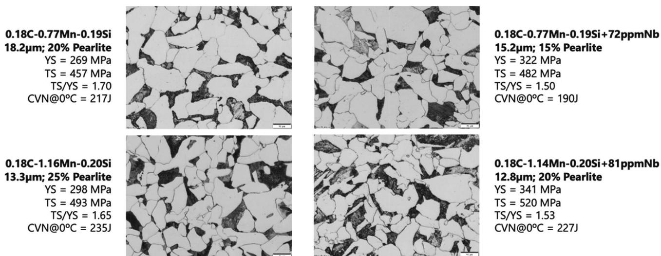
**Figure 5:** Comparison of the microstructures for the CMn (at left) and ULNb (at right) steels with 0.77 and 1.14% Mn at FRT of 950°C [1].
