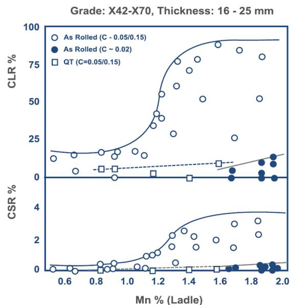
**Figure 10:** Effect of manganese content in steel on its susceptibility to hydrogen cracking, expressed in terms of crack length ratio (top graph) and crack sensitivity ratio (bottom graph) [12].
