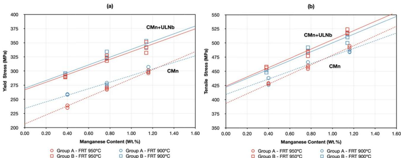
**Figure 4:** Effect of manganese content on (a) yield stress and (b) tensile stress) for CMn (Group A) and ULNb (Group B) steels, considering finish rolling temperatures of 950°C and 900°C [1].
