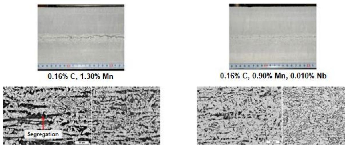
**Figure 3:** Effect of reducing manganese content in Q345 steel: (a) original Mn content; (b) reduced Mn, showing minimization of central segregation and greater uniformity of the microstructure of the final product [8].
