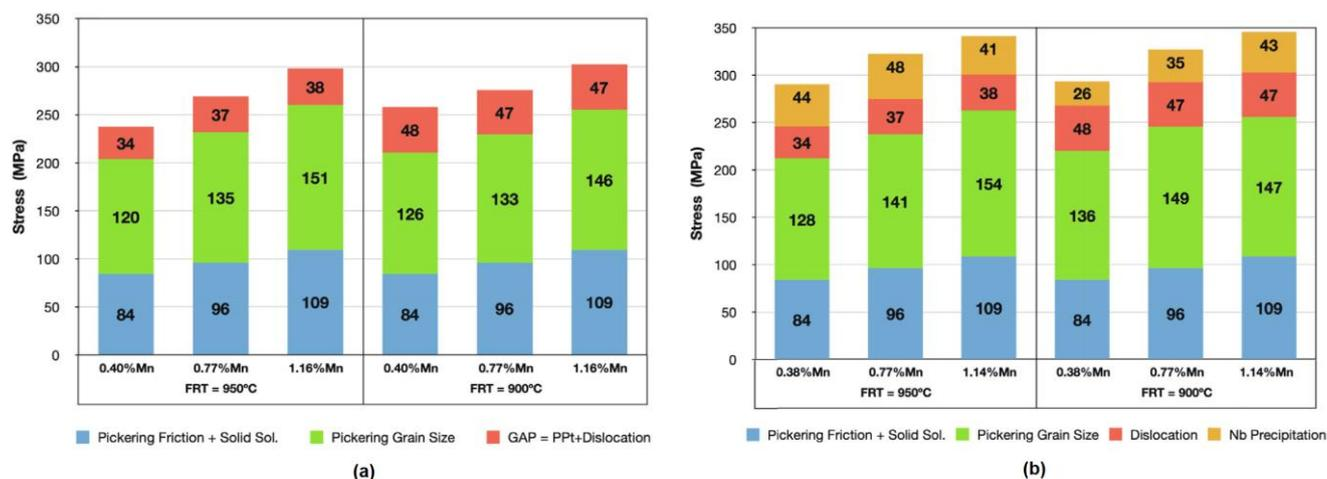
**Figure 7:** Breakdown of individual strengthening components for (a) Group A and (b) Group B steels [1].
