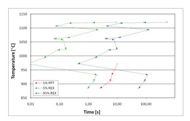
Figure 4: Curves for 5% and 95% austenite recrystallization and 5% NbCN precipitation determined by the Dutta-Valdes-Sellars model for a steel with 0.15% C and 0.015% Nb processed according to the heavier pass schedule.
