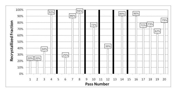
Figure 1: Prediction of the recrystallized fraction between consecutive passes during normalizing rolling of a C-Mn steel according to the default pass schedule described here.
