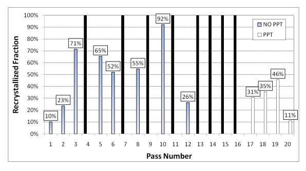
Figure 5: Recrystallized fraction predicted between passes during the normalizing rolling of a 0.15%C, 0.020% Nb and 0.0085% N steel according to the default pass schedule described here.
