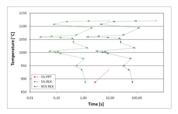
Figure 3: Curves for 5% and 95% austenite recrystallization and 5% NbCN precipitation determined by the Dutta-Valdes-Sellars model for a steel with 0.15% C and 0.015% Nb processed according to the default pass schedule.
