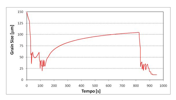
Figure 6: Grain size evolution predicted during normalizing rolling of a 0.15%C, 0.020% Nb and 0.0085% N steel according to the default pass schedule described here.
