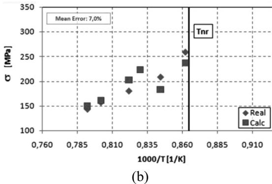
**Fig. 4:** MFS evolution along finishing mill for strips (a) #2A and (b) #2B.
