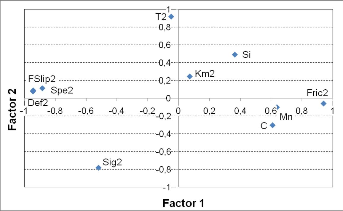
Figure 1: Results of the principal components analysis determined from F2 stand rolling data. Legend: **C**, carbon content; **Mn**, manganese content; **Si**, silicon content; **T2**, rolling temperature; **Def2**, strain degree, **Km2**, length of strip processed up to that moment by the work rolls; **FSli2**, forward slip; **Sig2**, hot strength; and **Fric2**, friction coefficient.
