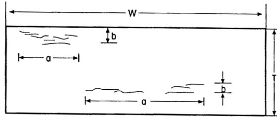
**Figure 7.** Test specimen and crack dimensions to be used for the calculation of CSR, CLR and CTR [12].
