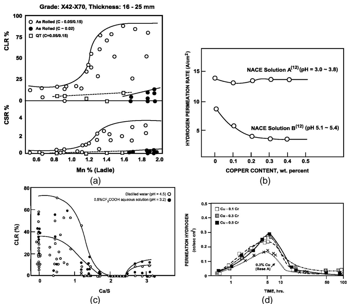
**Figure 4.** Effect of alloy elements on HIC: a) Mn; b) Cu; c) Ca/S ratio and d) Cr. CLR: crack length ratio; CSR: crack sensitivity ratio [4]. See Figure 7.
