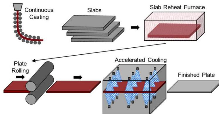
**Figure 2.** Schematic of thermomechanical controlled processing (TMCP) of plate [2].
