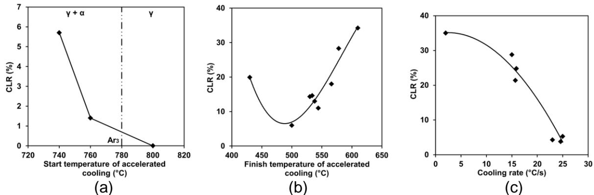
**Figure 6.** Effect of some parameters of accelerated cooling after plate rolling on HIC resistance [8]. CLR: crack length ratio, see Figure 7.
