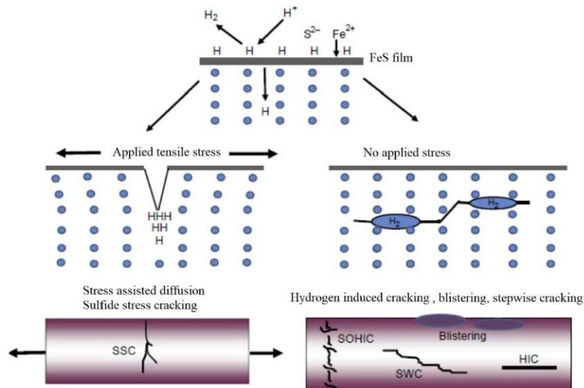
Figure 3. Formation of HIC and SSC cracks [3].
