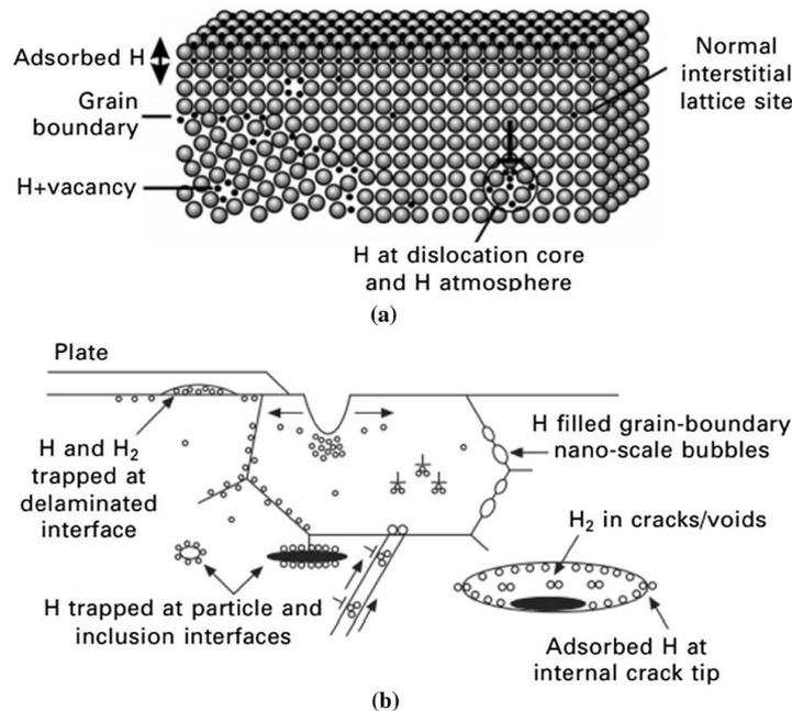
**Figure 5.** Trap sites for hydrogen in steels: a) on atomic scale; b) on microscopic scale [3].
