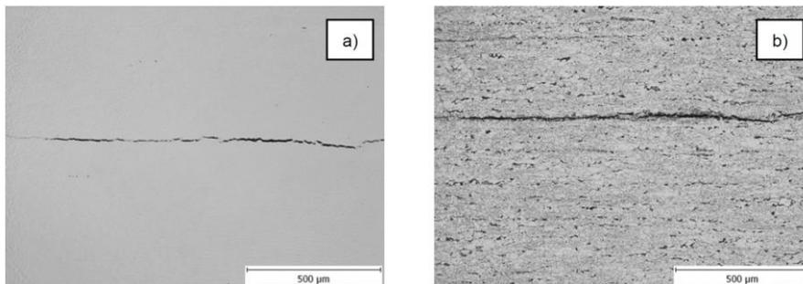
**Figure 7.** Typical cracks induced by H seen in the metallographic specimens of steel plates for pipes [11].
