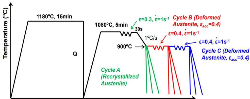
Figure 1. Thermal cycles performed to determine the CCT diagram.
