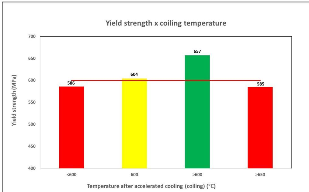
Figure 10. Yield strength x coiling temperature.
