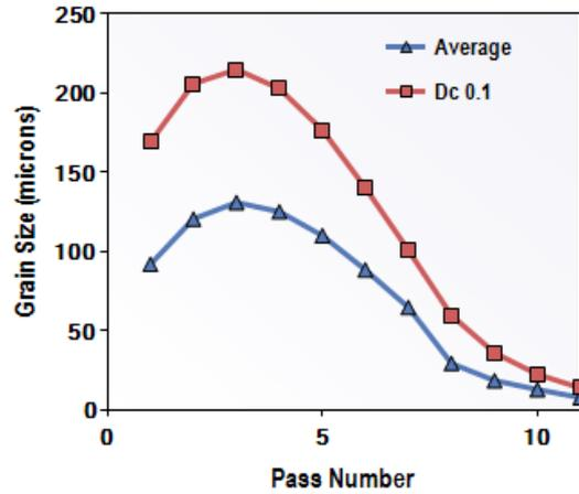
**Figure 6.** Simulations obtained via MicroSim-SM® for medium austenitic grain size and Dc01.
