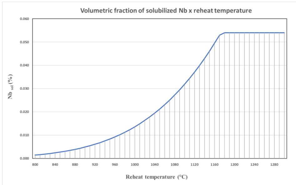
**Figure 3:** Reheating temperature x volumetric fraction of solubilized Nb for the steel under study, as predicted by Irvine [12].
