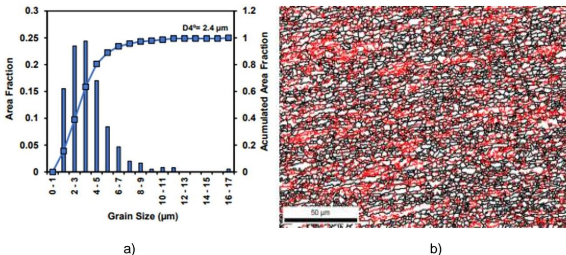
**Figure 8.** a) Ferritic grain size distribution obtained in one of the rolled strips b) Image of the microstructure obtained via SEM-EBSD of the rolled strip.
