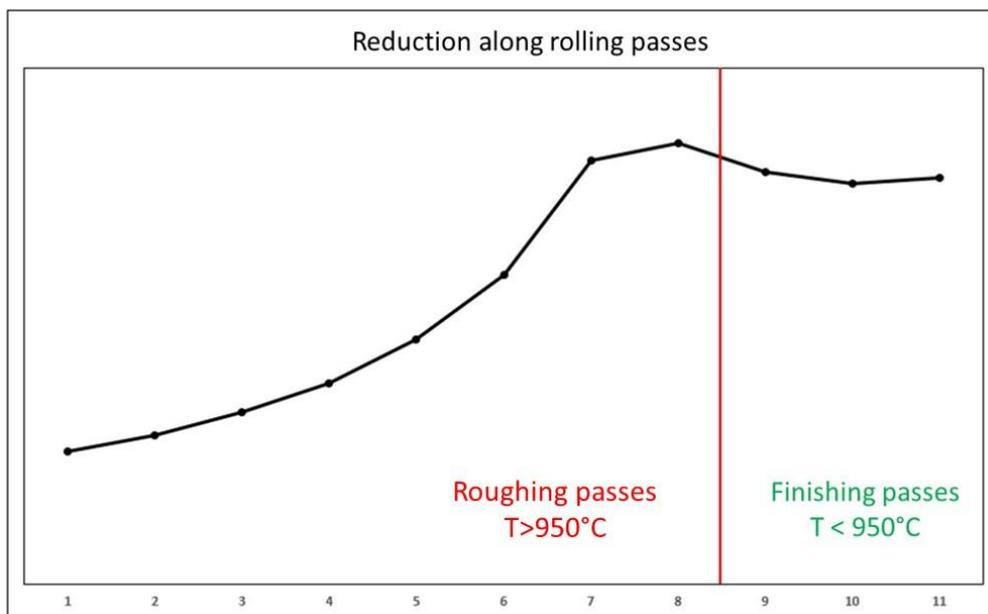
**Figure 5.** Reduction percentage during the rolling process.
