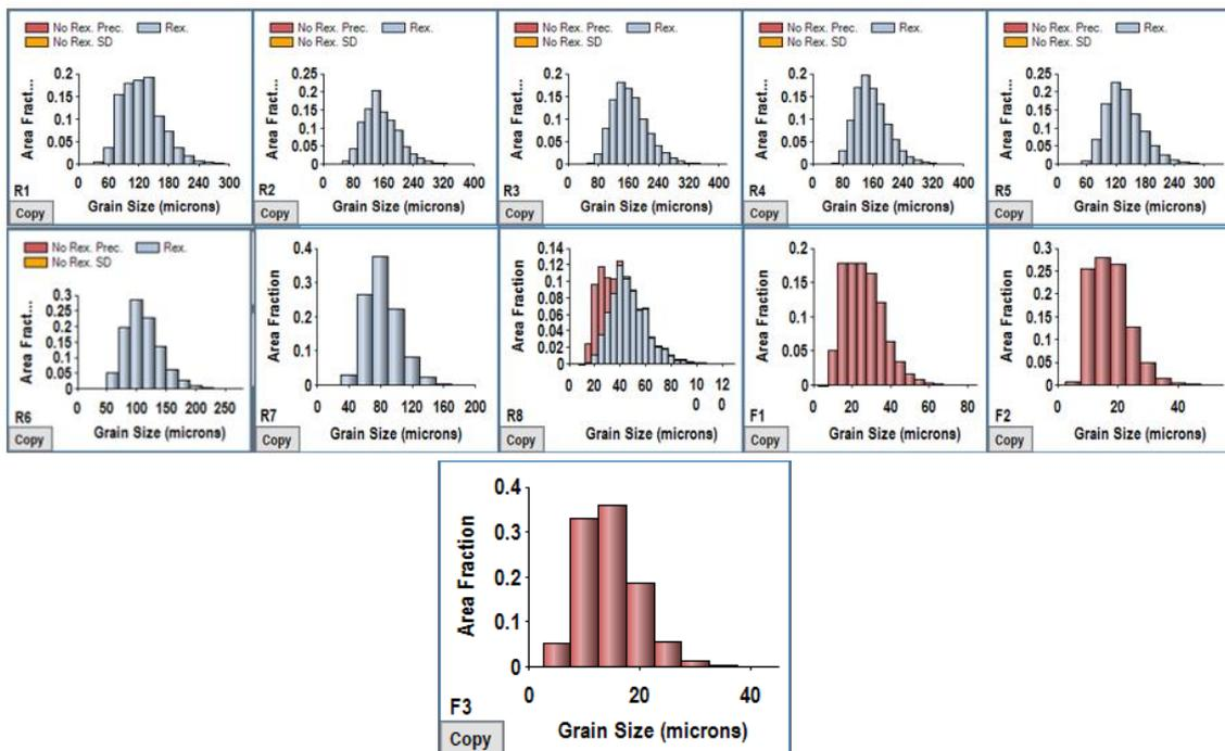
**Figure 7.** Evolution of austenitic grain size distribution per pass predicted by MicroSim-SM®.
