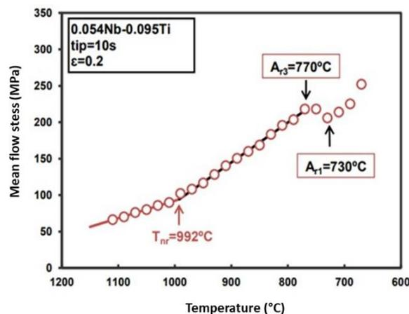
**Figure 2.** Mean flow stress curve versus temperature obtained through hot torsion tests for the steel under study - T<sub>nr</sub> (992°C), Ar<sub>3</sub> (770 °C) e Ar<sub>1</sub> (730 °C).
