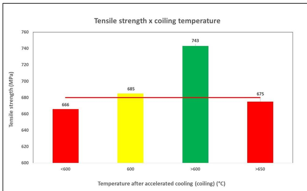
Figure 11. Tensile strength x coiling temperature.
