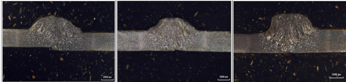
(Sample 1) CMn x CMn (Sample 2) ULNb x ULNb (Sample 3) CMn x ULNb Figure 1: Macrographs of the welded joints made with high welding energy.
