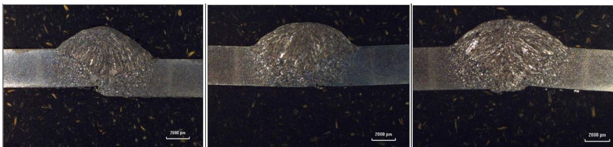
(Sample 4) CMn x CMn (Sample 5) ULNb x ULNb (Sample 6) CMn x ULNb Figure 2: Macrographs of the welded joints made with standard energy.
